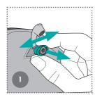
Pull the valve ring upwards. Move it to the side until the vacuum cushion becomes soft.
