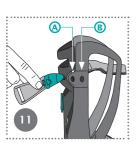
Push the buckle out of the lower shell and into the desired position.
