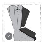
Stroke the fabric liner smooth to distribute the small spheres evenly.
